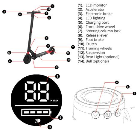
(1). Acceleration / brake gauge / errors indicator (2). Battery level indicator (3). Lights indicator (4). Speed - and ON/OFF lights button (5). ON/OFF device button
